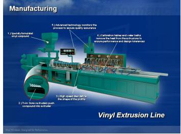
For use as window profiles, the specially-formulated resin, augmented with processing additives and pigments, must be processed into final form through an extrusion process. In this step, the resin is melted and the resulting soft mass is forced through dies that give it its final shape. The extrusions are cooled under carefully controlled conditions to ensure that intended shapes and tolerances are maintained.
